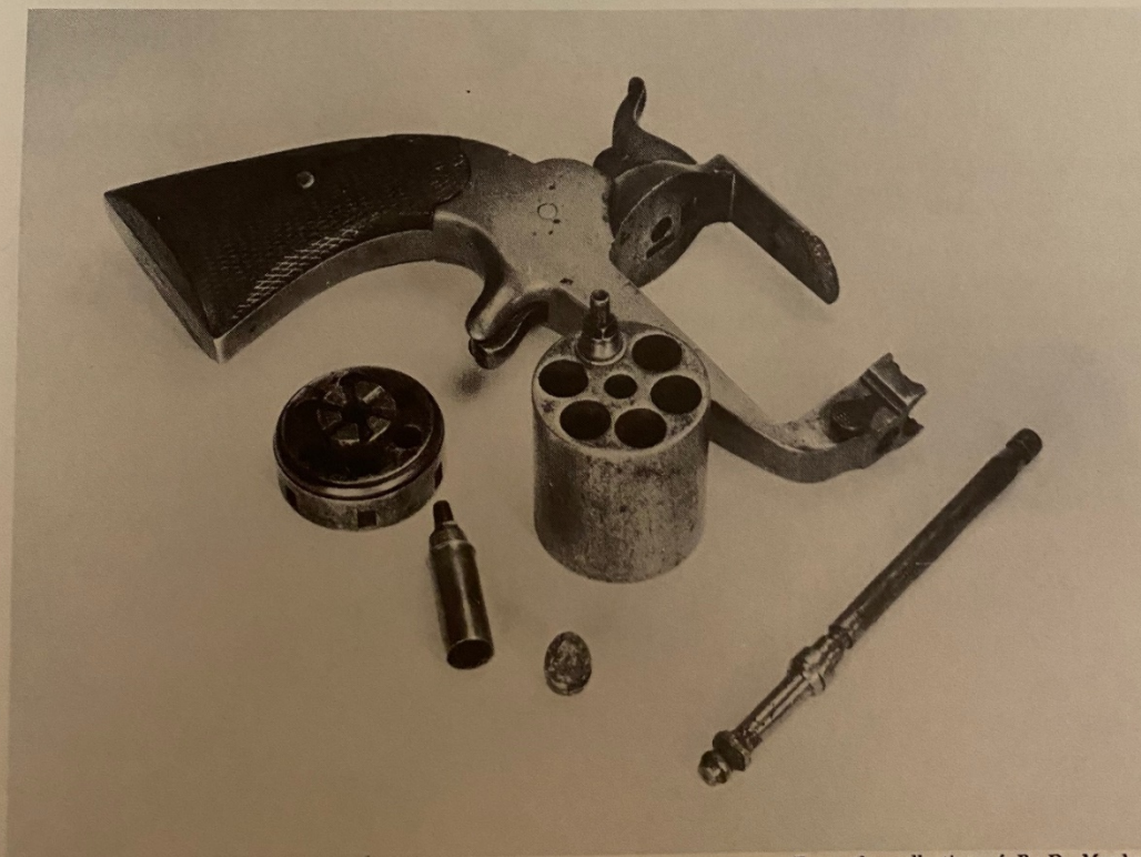
PLATE 24A. 1st Model of the Cofer revolver, showing the 2 picced cylinder, and the special cartridge required.
