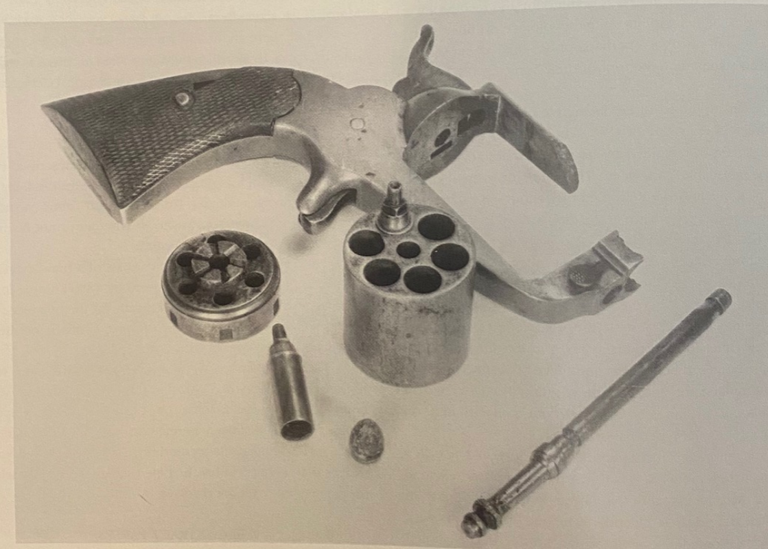
Patented two-piece or split-cylinder percussion-cartridge revolver. Ser. No. 7. Exploded view of remnant revolver depicting component parts. Two known examples.
